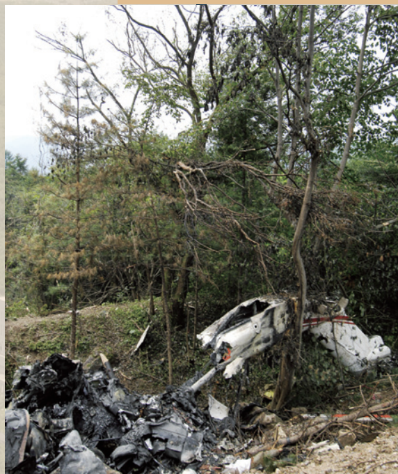
The tail of the helicopter was miraculously caught in a Y-shaped tree as it came down, so the craft could not spin around.
